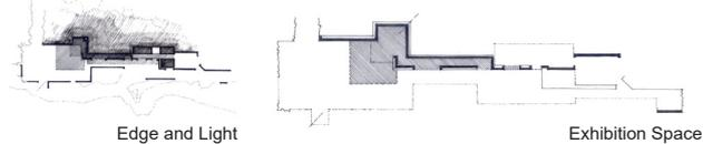
**Precinct Edges:** The berm edge into which the facilities are tucked establishes a robust structure of rough off-shutter concrete and packed stone walls. The concrete overhead shelf allows this wall edge to be sheltered and protected. The wall to the forecourt retains the vegetated embankment and is defined in accommodating a series of functions along its length.
